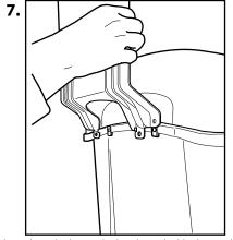
Align the 2 holes with the threaded holes in the metal brackets attached to the bin rear. **Notes:** Do not place sign holder into cutout slots on bin rim. Sign can only be fitted at the rear of the bin.
