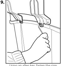
Using an allen key, fasten the sign holder to the bin securely.
