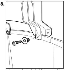
Arrange the included fixtures as follows; Screw, Washer, Locking Washer.
